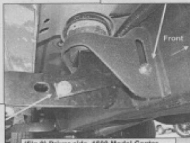
(Fig 9) Driver side, 1500 Model Center Bracket and Support Bracket Installation
