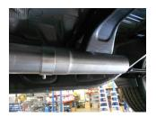
2) If installing the system on a Crew Cab truck with a 6.5' bed, place extension pipe **#TB700S** onto the back of the **#26409S** inlet pipe, place a provided clamp onto the slip-fit and tighten enough to hold in position. This extension pipe will not be used on Double Cab or Crew Cab-5.5' bed models.
