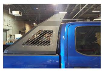
**STEP 7**// Place the Chase Rack on top of the bed rails. Be sure to center the rack. Adjust the Chase Rack forward or backwards so that the rack does not make contact with the truck cab.
