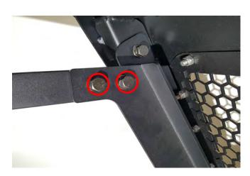
STEP 4 // Install both driver and passenger side vertical support braces using the (2) 10 x 25mm bolts, flat washers, and lock washers.
