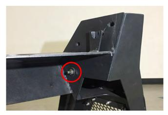
**STEP 1** // Connect the middle light tray to the driver side upright using (1) M10 x 35mm bolts, and (1) M10 nuts, and (2) M10 flat washers, and (1) M10 lock washers.
