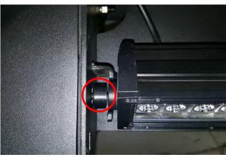
**STEP 9**// Light bar must be installed prior to installing the upper mesh cover. Insert the M8 x 40mm bolts, lock washers, and flat washers through the upright and light tray. Install the provided spacers between the light bar and the tray as seen above. Do to the differing widths of 40" light bars, additional 2.5mm spacer/washers are included.
