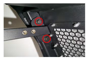
**STEP 2** // Install the horizontal rack support brace using (2) M10 x 25mm bolts, flat washers, and lock washers.
