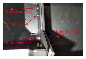
**STEP 6**// Insert the dual nut plate through the hole in the middle light tray. Using the tab on the nut plate align the bolt holes. Install the (1) M10 x 35mm bolts, lock washers, and washers through the outside of the upright and into the dual nut plate. This will tighten the mesh grille cover to the top of the chase rack. Repeat on other side.
