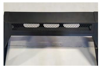
**STEP 5** // If installing the optional light bar, refer to Step 9 before continuing. Place the upper mesh cover between the uprights.
