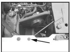
Step 12 Remove the bolt shown and rotate the brace towards the engine.
