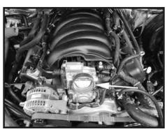
Step 15 Install the throttle body adapter ring onto the throttle body.
