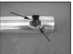
Step 8 Insert and fasten the MAFS onto the intake tube with the provided machine screws.
