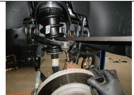
Lift suspension slightly while prying down to attach ball joint.
