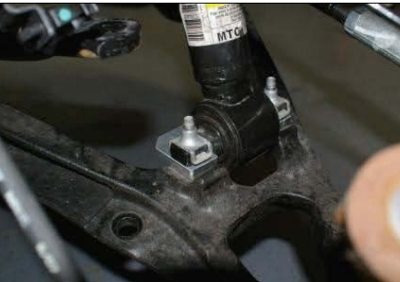
Image: Spacer installed
