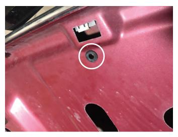
Press the well nuts into the factory holes. If the holes are slightly oversized, use tape to hold well nut in place. \*\*Note: If tape is used the hole in the well nut needs to remain open.
