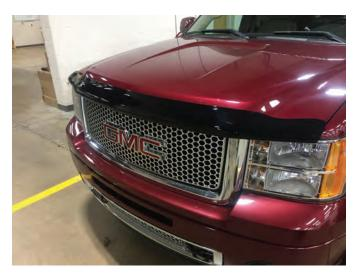
Hold the Bug Deflector up to the hood. Tighten the supplied screws into the well nuts. \*\*Note: if the well nut doesn't tighten, you may need to apply firm pressure on the Bug Deflector to prevent the well nut from spinning in the hole. Once the well nut tightens up it will stop spinning in place.
