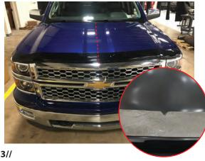
Before removing the tape backing, test fit the Bug Deflector on the hood. Center the Bug Deflector on the hood using the factory body line and the notch in the Bug Deflector as a reference points. \*\*Note the location of the metal clips for the next step.
