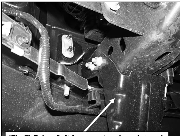
(Fig 7) Driver/left frame extension pictured
