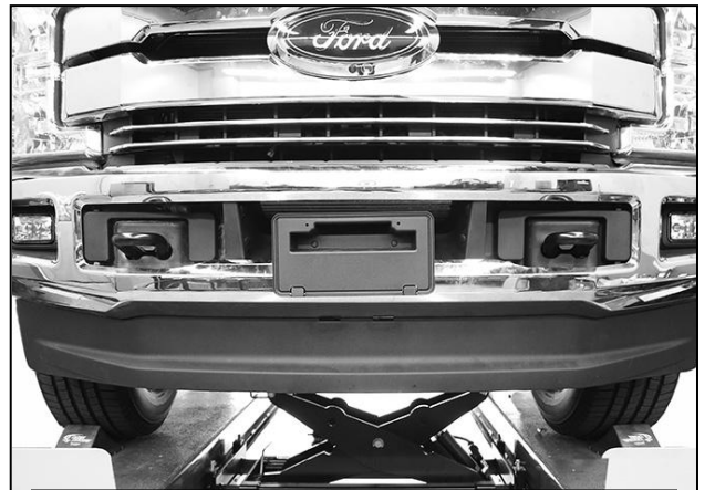
(Fig 6) Remove plastic air dam from bumper
