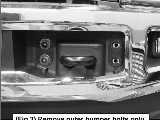
(Fig 3) Remove outer bumper bolts only
