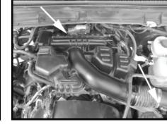
**Disconnect the crank case vent**
