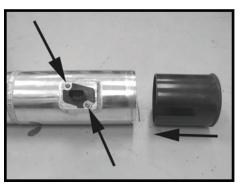
Step 8 Install the MAFS into the SR Performance aluminum intake tube, then install the MAFS Sleeve into the aluminum intake tube.
