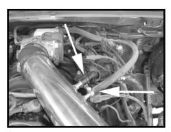
Step 14 Reconnect the crank case vent line and using the supplied mini clamp fasten the EVAP to nipple on the intake tube.
