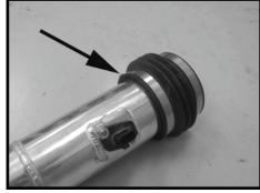
Step 9 Install the flex coupler onto the intake tube and secure with the provided hose clamp. Install a second clamp but do not tighten at this time.
