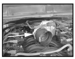
Step 12 Install the angled coupler on the throttle body and secure the coupler in place.
