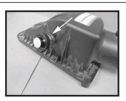
Step 6 Remove the filter minder and grommet from the air box lid.
