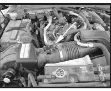
Step 4 Loosen the clamp on the air box lid from the factory intake tube. Remove the air box lid and filter from the vehicle.
