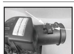
Step 5 Remove the 2 screws securing MAFS from the air box lid. Then remove the sensor from the air box.
