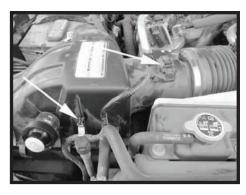
Step 2 Slide the red clip back then disconnect the electrical connector at the Mass Air Flow Sensor (MAFS). Unclip the wiring harness from the air box lid.
