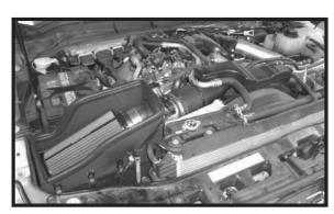
Step 11 Reconnect the battery cable, start the vehicle and let it warm up. Shut off and inspect the installation once more for any loose clamps, wires, or hardware. Test drive & enjoy! Your installation is now complete. Periodically check all clamps and brackets.
