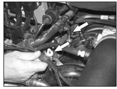
30c. Re-install the heater control valve and wiring harness mounting clips onto the air box mounting studs as shown.
