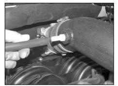
30. Install the provided silicone vent hose onto the valve cover and onto the K&N $^{\circ}$  intake tube as shown.
