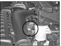
5. Remove the intake tube mounting bolt shown.
