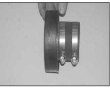
32. Install the silicone hose (#08630) onto the K&N<sup>®</sup> filter adapter and secure with the provided hose clamp as shown.
