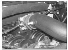
27. Install the K&N<sup>®</sup> intake tube into the silicone hose and then tighten the provided hose clamp.
