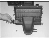
19. Remove the two screws that secure the mass air sensor to the air box with the provided wrench, then remove the mass air sensor.
