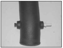
24a. On vehicles that are equipped with only one vent line, install the provided NPT plug as shown.
