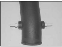
24. Install the provided NPT fittings into the intake tube as shown.
