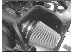
34. Install the K&N<sup>@</sup> air filter assembly onto the K&N<sup>@</sup> intake tube as shown and secure with the provided hose clamp.
