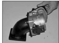
12. Using the bolts removed in step #10, secure the throttle body to the K&N<sup>®</sup> throttle body adapter with the gasket as shown.
