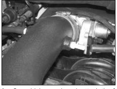
30a. On vehicles equipped, attach the factory brake booster vent hose to the K&N $^{\mbox{\tiny ®}}$  intake tube as shown.
