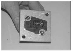
21. Install the mass air sensor into the K&N<sup>®</sup> mass air adapter as shown and secure with the provided hardware.
