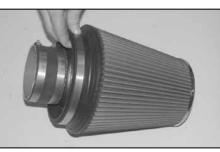
33. Install the adapter assembly into the K&N $^{\ensuremath{\mathbb{R}}}$  air filter as shown.
