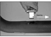
22. Install the mass air sensor assembly into the  $K\&N^{\circledast}$  intake tube.
