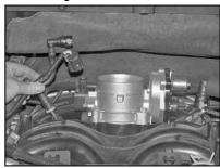
9. Disconnect the TPS sensor electrical connection from the throttle body.
