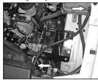
17b. Install the supplied coolant recovery hose and secure with the provided hose clamps. **NOTE: Be sure to replace the coolant that was recovered during hose removal by replenishing it in the coolant recovery tank.**
