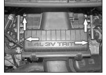
4. Remove the four air box mounting bolts shown
