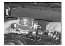
11. Lift the throttle body from the intake manifold and disconnect throttle body motor electrical connection.
