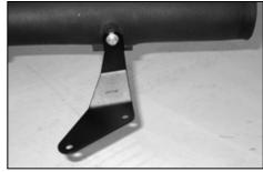
25. Install the tube mounting bracket (070118) onto the K&N $^{\circ}$  intake tube as shown with the provided hardware.
