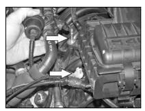
3b. Pull up on the heater control valve and wiring harness mounting clips to unhook them from the air box mounting studs as shown.
