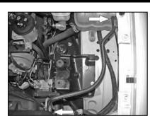
17a. Loosen the coolant recovery hose, hose clamps, and then remove the factory recovery hose shown. Be sure to catch any coolant, which flows out of the radiator during hose removal. **NOTE: Be sure to let the engine cool completely before removing the overflow hose or hot coolant will escape from the radiator and injury or damage may result.**
