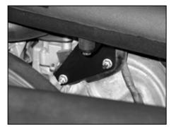
28. Connect the K&N $^{\mbox{\tiny \$}}$  intake tube to the bracket with the provided hardware as shown.
