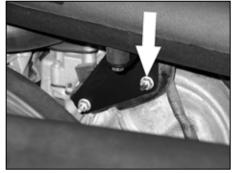
28a. On vehicles not equipped with the factory intake tube support bracket, it is necessary to use the supplied 8mm bolt, washers and nut to secure the tube mounting bracket to the engine bracket as shown.
