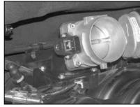
13. Install the throttle body assembly onto the intake manifold with the hardware provided as shown.
