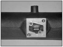
23. Secure the mass air sensor assembly onto the K&N $^{\odot}$  intake tube with the provided hardware as shown.
