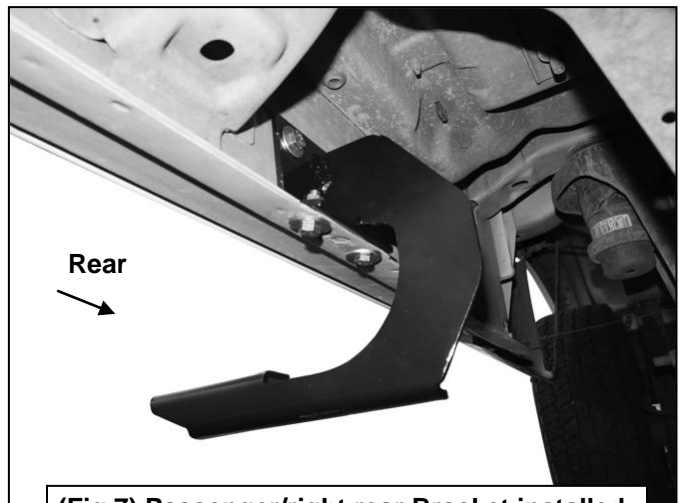
(Fig 7) Passenger/right rear Bracket installed
