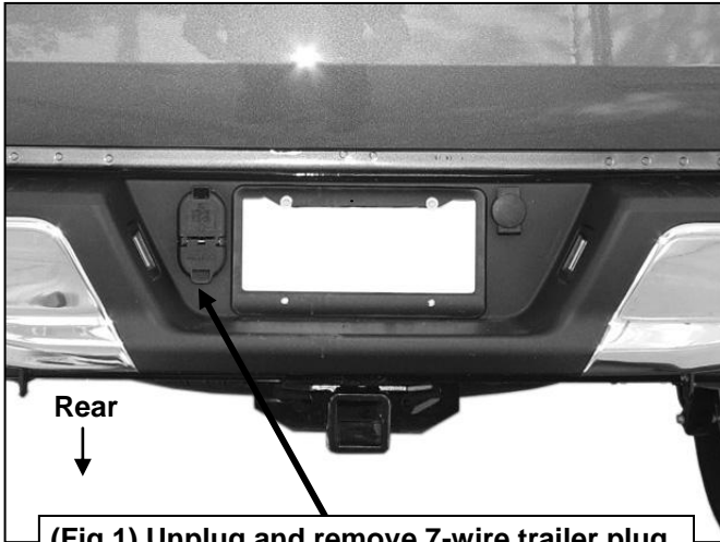
(Fig 1) Unplug and remove 7-wire trailer plug
