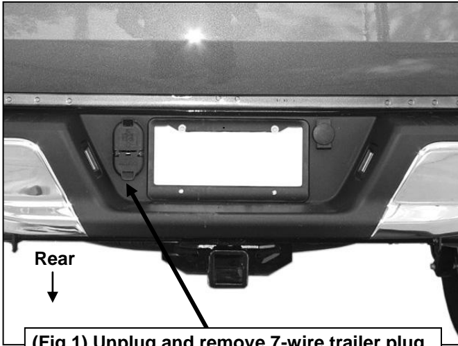
(Fig 1) Unplug and remove 7-wire trailer plug
