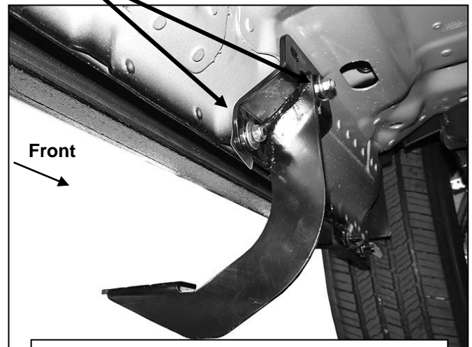
(Fig 4) Driver side front Bracket installation
