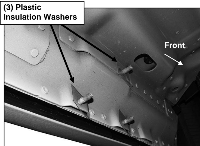
(Fig 3) Thread Plastic Washers onto all mounting studs. Driver side front location pictured
