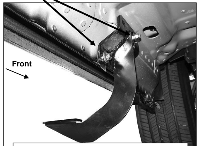
(Fig 4) Driver side front Bracket installation
