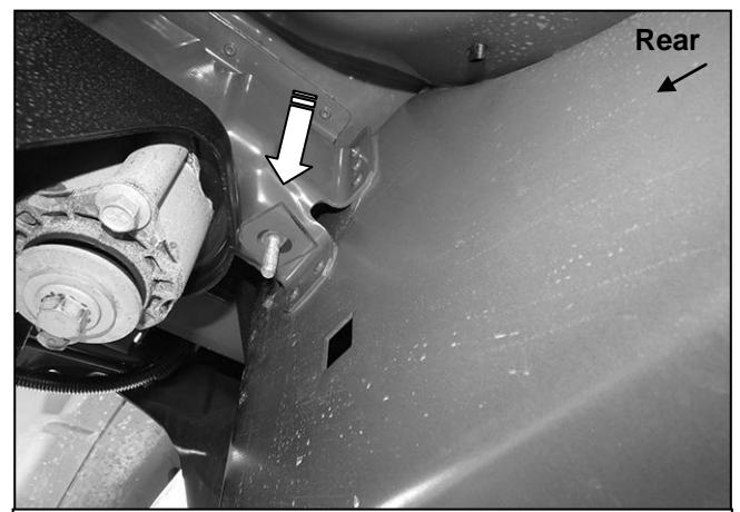
(Fig 10) Insert T-Bolt and folded Washer into oval hole. Thread second Plastic Washer onto T-Bolt
