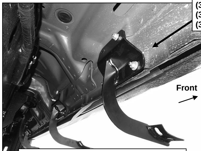
(Fig 5) Driver side front bracket installed
