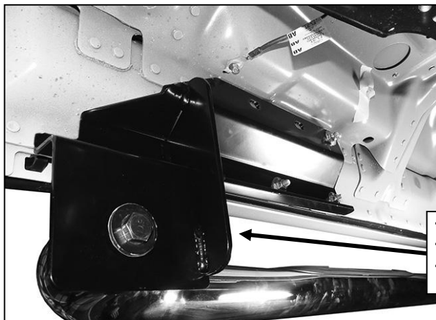
(Fig 5) Passenger side front Bracket installation
