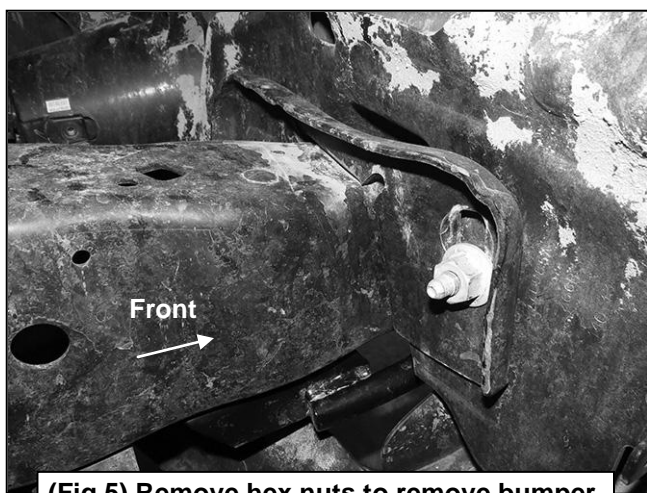
(Fig 5) Remove hex nuts to remove bumper
