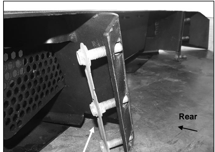
(Fig 4) On models without receiver hitch, reuse triple bolt plate to attach bumper to ends of frame
