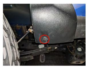
**STEP 11** // Lay the fender flare against the wheel well, from the bottom up insert the (1) push pin securing the bottom of the flare to the vehicle.
