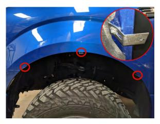
**STEP 5** // Install the (3) mounting brackets to the wheel well using the factory screws. \*\*Note, do not fully tighten the screws.
