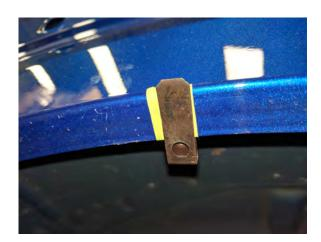
**STEP 10** // Insert the (4) body clips on the lip of the wheel well over the tapped locations from the inside out. \*\*Note If you have factory flares, clips will not line up with the factory holes.
