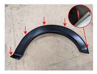
**STEP 1** // Begin by installing the supplied rubber edge trim onto each fender flare where the flare meets the body of the vehicle. Peel back approx 2" of the red lining, and push the rubber trim onto the edge of the flare that meets the body of the vehicle. Then completely pull the red backing off and firmly press the trim to bond to the flare. Cut the trim to length. \*\*Note, rubber trim covers end to end.
