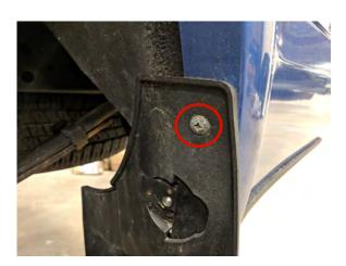
**STEP 3** // If your vehicle is equipped with factory fender flares and mud flaps they must be removed before installation of the Barricade flares.
