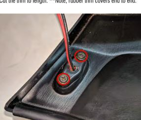
**STEP 2** // Install the LED marker light to the flare. Insert the two wires through the center hole, and secure the light to the flare using the (2) 8mm x 1/2 screws.
