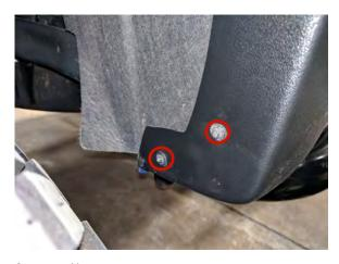
**STEP 7** // While pushing the flare flush against the wheel well, install the (2) factory screws in the front, and the (2) factory screws on the rear to secure the flare to the vehicle. \*\*Note, fully tighten the mounting brackets from Step 5 once the flare is fully flush against the body of the vehicle.
