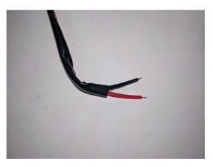
**STEP 8**// Install the supplied wiring harness to the marker light on each fender flare and tap the Red 12v + wire and Black - wire into the driver side marker light harness.
