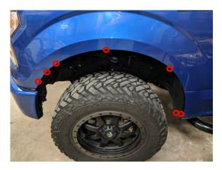
**STEP 4 // Front Fender Flares:** Locate, and remove the factory (7) 5.5mm screws. \*\*Note factory screws will be reused.
