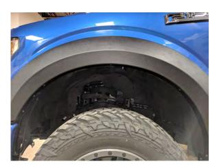
**STEP 6** // Attach the front fender flare marked (D) to the mounting brackets using the (3) 8mm x 1/2 screws. \*\*Note, leave the wires for the marker light facing out from the fender flare.
