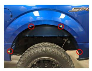
**STEP 9** // **Rear Fender Flares:** With a helper, hold the rear fender flare marked (D) tight against the wheel well. Using painters tape, mark the locations on the lip of the wheel well were the body clips are going to mount by matching up with the holes of the fender flare.
