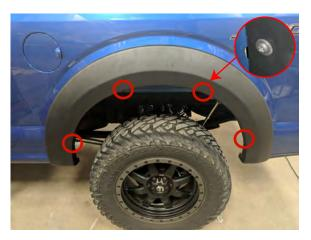
**STEP 12** // Install the fender flare to the wheel well body clips using the (4) 8mm x 3/4 screws. Do not over-tighten. Installation is now complete. \*\*Note, push in on the fender flare where needed to reduce fender gaps.
