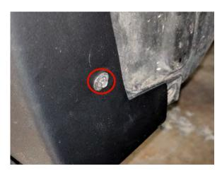
**STEP 7** // While pushing the flare flush against the wheel well, install the (1) factory screw in the bottom rear to secure the flare to the vehicle. \*\*Note, fully tighten the mounting brackets from Step 5 once the flare is fully flush against the body of the vehicle.
