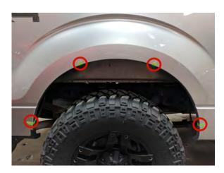
**STEP 9** // **Rear Fender Flares:** With a helper, hold the rear fender flare marked (P) tight against the wheel well. Using painters tape, mark the locations on the lip of the wheel well were the body clips are going to mount by matching up with the holes of the fender flare.
