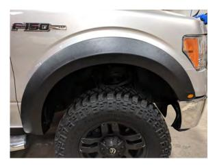
**STEP 6** // Attach the front fender flare marked (P) to the mounting brackets using the (3) 8mm x 1/2 screws. \*\*Note, leave the wires for the marker light facing out from the fender flare.
