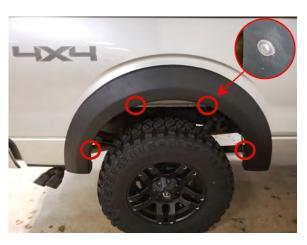
**STEP 11** // Install the fender flare to the wheel well body clips using the (4) 8mm x 3/4 screws. Do not over-tighten. Installation is now complete. \*\*Note, push in on the fender flare where needed to reduce fender gaps.
