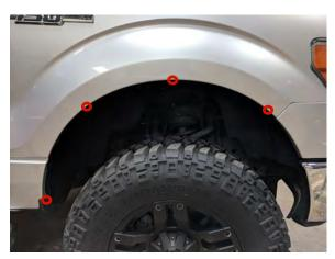
**STEP 4 // Front Fender Flares:** Locate, and remove the factory (4) 5.5mm screws. \*\*Note factory screws will be reused.
