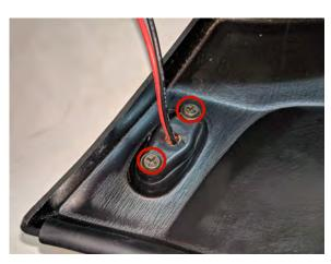
**STEP 2** // Install the LED marker light to the flare. Insert the two wires through the center hole, and secure the light to the flare using the (2) 8mm x 1/2 screws.
