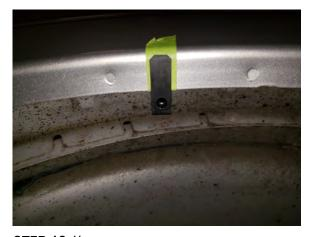
**STEP 10** // Insert the (4) body clips on the lip of the wheel well over the tapped locations from the inside out. \*\*Note If you have factory flares, clips will not line up with the factory holes.
