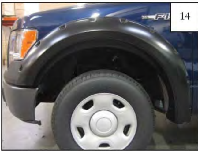
Completed front flare installation.
