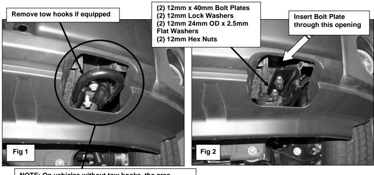
NOTE: On vehicles without tow hooks, the area circled above may be covered by an indented plastic panel. Cut or remove the panel as required to gain access to the front of the frame rail to allow bottom brackets to pass through the bumper cover.
