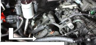
21" Hose with 45 degree fitting to intake manifold
