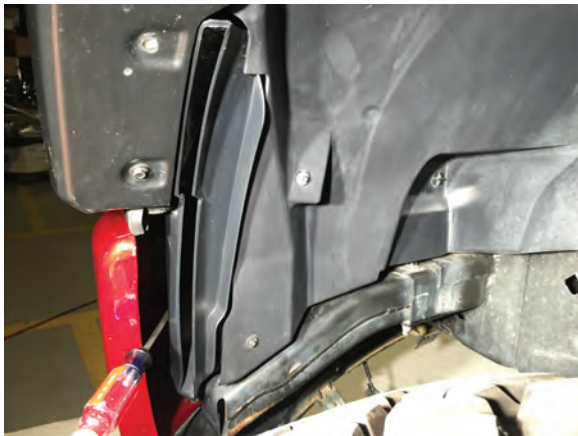
Step 4 It may be necessary to pry on the less accessible side of the fog light housing. Using a long flat blade screwdriver you can pry the housing from the wheel well as seen above, or you can loosen/ remove the fender liner for better accessibility.
