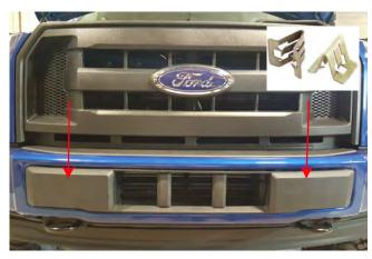
**STEP 1** // Using a panel removal tool, remove the plastic bumper insert. It is held in with several metal push clips.
