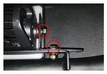
**STEP 5** // If purchased with the LED lighting option, install the LED light using the hardware provided in the light packaging. If choosing not to use the LED lighting. The bumper will include a bolt on mesh cover. Secure the cover to the bumper using (4) M8 x 20mm bolts, lock washers, and nuts.
