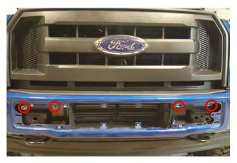
**STEP 2** // Next, loosen the upper (4) 21mm nuts holding the front bumper to the support beam of the vehicle. \*\*Note: Factory hardware will be reused.
