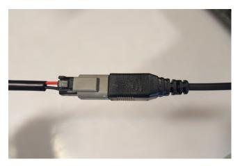
**STEP 8** // Optional LED light wiring, connect the (2) LED lights into the supplied harness. Be sure to zip tie the access wiring away from any damage that could occur.
