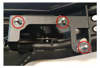
**STEP 6** // Using the supplied (6) plastic washers attach the factory bolts to the RedRock 4x4 bumper.
