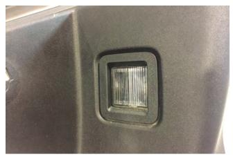
**STEP 5** // Using a flat head screw driver, push in the plastic tabs around the license plate lights, and remove it from the factory bumper. Install these in the new Barricade bumper by pushing them in place till they snap in.
