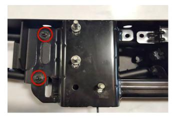
**STEP 7** // If your vehicle is equipped with a factory trailer hitch receiver, remove the (10) factory M10 bolts from the factory bumper. Install the hitch receiver to the Barricade bumper using the (2) double bolt plate, (4) M10 lock nuts, and (4) M10 flat washers.
