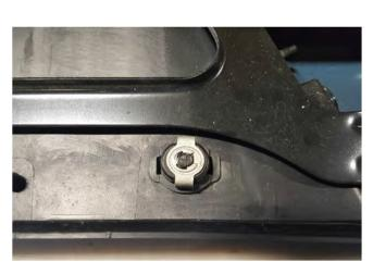
**STEP 4** // Using your factory ignition key, turn the spare tire lock clockwise and remove the spare tire lock from the factory bumper. Then install it in the new Barricade bumper.
