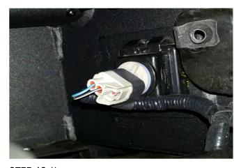
**STEP 10** // Plug the factory license plate lights harness and the trailer plug connector back in.
