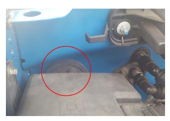
**STEP 13** // Optional LED light wiring, route the on/off switch to the interior of the vehicle using a suitable body grommet. Mount the switch in the desired location. Zip tie any extra loose wiring away from any damage that could occur.
