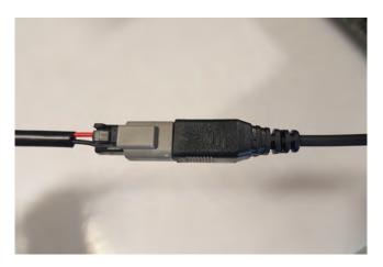
**STEP 11** // Optional LED light wiring, connect the (2) LED rock lights into the supplied harness. Be sure to zip tie the access wiring away from any damage that could occur.
