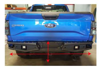
**STEP 9** // Attach the new Barricade bumper to the vehicle using the factory (6) 21mm nuts. Be sure to center the bumper, and adjust height of bumper to desired location.
