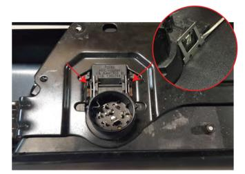
**STEP 3** // Using a flat head screw driver, push in the metal tabs around the trailer plug connector and remove it from the factory bumper. Reinstall the trailer plug into the new bumper. If it does not clip in, use a small screw driver to expand the clips.
