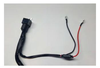
**STEP 12** // Optional LED light wiring, install the Red 12 + volt wire to the positive battery terminal. Connect the black ground wire to the negative battery terminal. Mount the fuse in a safe location away from any damage that could occur. Tuck away any extra wiring.
