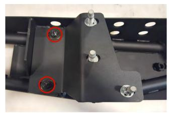
**STEP 8** // If your vehicle is not equipped with a trailer hitch receiver, install the two mounting brackets to the bumper using the (2) double bolt plate, (4) M10 lock nuts, and (4) M10 flat washers.
