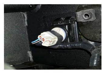
**STEP 11** // Plug the factory license plate lights harness and the trailer plug connector back in. Plug in all factory electrical connections included the license plate lights, trailer plug, and if equipped the reverse sensors.
