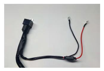
**STEP 13** // Optional LED light wiring, install the Red 12+ volt wire to the positive battery terminal. Connect the black ground wire to the negative battery terminal. Mount the fuse in a safe location away from any damage that could occur. Tuck away any extra wiring.
