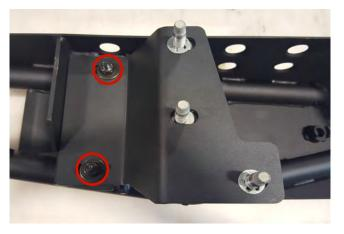
**STEP 8** // If your vehicle is not equipped with a trailer hitch receiver, install the two mounting brackets to the bumper using the (2) double bolt plate, (4) M10 lock nuts, and (4) M10 flat washers.
