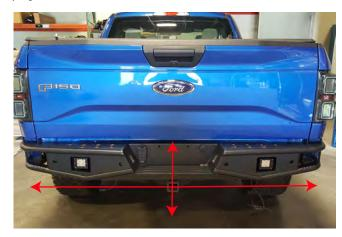
**STEP 10** // Attach the new RedRock 4x4 bumper to the vehicle using the factory (6) 21mm nuts. Be sure to center the bumper, and adjust height of bumper to desired location.
