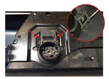
**STEP 3** // Using a flat head screw driver, push in the metal tabs around the trailer plug connector and remove it from the factory bumper. Reinstall the trailer plug into the new bumper. If it does not clip in, use a small screw driver to expand the clips.
