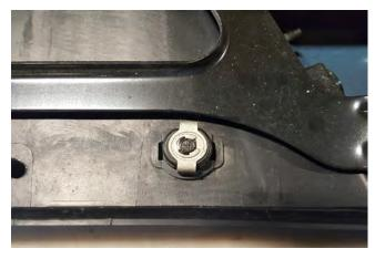
STEP 4 // Using your factory ignition key, turn the spare tire lock clockwise and remove the spare tire lock from the factory bumper. Then install it in the new RedRock 4x4 bumper.
