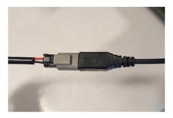
**STEP 12** // Optional LED light wiring, connect the (2) LED rock lights into the supplied harness. Be sure to zip tie the access wiring away from any damage that could occur.
