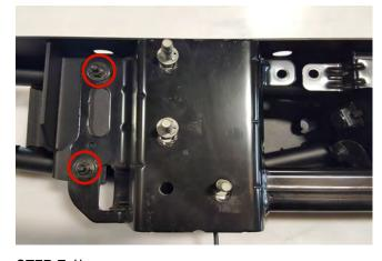
**STEP 7** // If your vehicle is equipped with a factory trailer hitch receiver, remove the (10) factory M10 bolts from the factory bumper. Install the hitch receiver to the RedRock 4x4 bumper using the (2) double bolt plate, (4) M10 lock nuts, and (4) M10 flat washers.
