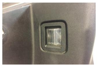
**STEP 5** // Using a flat head screw driver, push in the plastic tabs around the license plate lights, and remove it from the factory bumper. Install these in the new RedRock 4x4 bumper by pushing them in place till they snap in.
