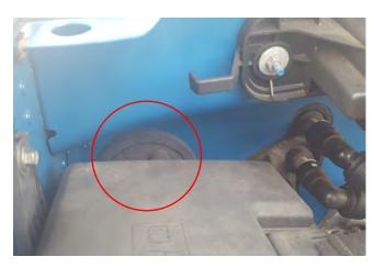
**STEP 14** // Optional LED light wiring, route the on/off switch to the interior of the vehicle using a suitable body grommet. Mount the switch in the desired location. Zip tie any extra loose wiring away from any damage that could occur.
