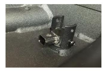
**STEP 9** // If equipped re-install the factory reverse sensors w/ the rubber grommet flush to the outer face of the bumper.
