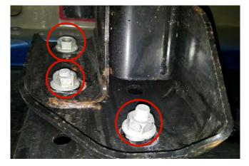
**STEP 2** // Remove the (6) 21mm nuts that hold the bumper to the frame rail. Remove bumper from vehicle. \*\*Note Factory 21mm nuts will be reused.
