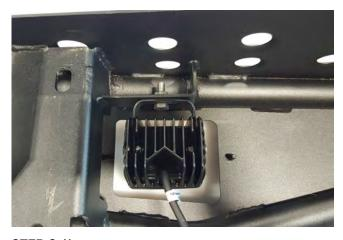
**STEP 6** // Optional LED lighting, install the LED lights using the hardware provided in the light packaging. If choosing not to use the LED lighting. The bumper will include bolt on mesh covers. Secure the cover to the bumper using the provide (2) M6 nuts and flat washer.
