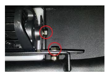
**STEP 4** // If purchased with the LED lighting option, install the LED light using the hardware provided in the light packaging. If choosing not to use the LED lighting. The bumper will include a bolt on mesh cover. Secure the cover to the bumper using (4) M8 x 20mm bolts, lock washers, and nuts.
