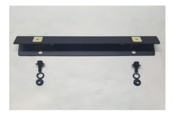
**STEP 3** // Attach the front license plate bracket to the new RedRock 4x4 bumper if a front license plate is required using the (2) M6 screws, lock washers, and nuts.
