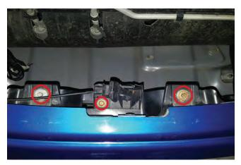
**STEP 1** // Remove the (2) 8mm screws, and (1) 10mm bolt that hold the hood latch plate to the factory bumper lip.
