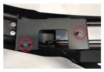
**STEP 5** // Using the supplied (4) plastic washers attach the factory bolts to the RedRock 4x4 bumper.
