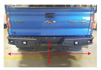
**STEP 8** // Attach the new RedRock 4x4 bumper to the vehicle using the factory (6) 21mm nuts. Be sure to center the bumper, and adjust height of bumper to desired location.
