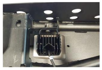
**STEP 5** // If purchased with the LED lighting option, install the LED lights using the hardware provided in the light packaging. If choosing not to use the LED lighting. The bumper will include bolt on mesh covers. Secure the cover to the bumper using the provide (2) M6 nuts and flat washer.
