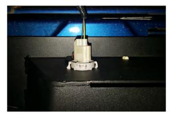
**STEP 9** // Plug the factory license plate lights harness and the trailer plug connector back in.
