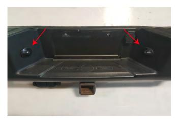
**STEP 4** // Using a flat head screw driver, push in the plastic tabs around the license plate lights, and remove it from the factory bumper. Install these in the new RedRock 4x4 bumper by pushing them in place till they snap in.
