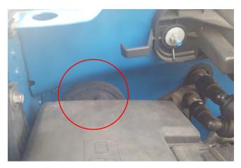
**STEP 12** // If purchased with the LED lighting option, Route the on/off switch to the interior of the vehicle using a suitable body grommet. Mount the switch in the desired location. Zip tie any extra loose wiring away from any damage that could occur.
