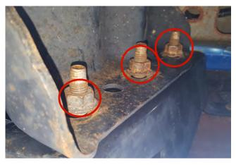
**STEP 2** // Remove the (6) 21mm nuts that hold the bumper to the frame rail. Remove bumper from vehicle. \*\*Note Factory hardware will be reused.
