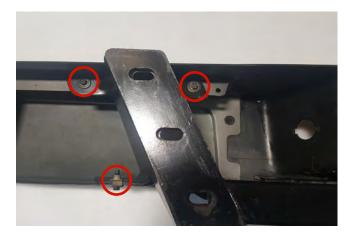
**STEP 6** // If your vehicle is equipped with a factory trailer hitch receiver, remove the (6) factory M8 bolts from the factory bumper. Install the hitch receiver to the RedRock 4x4 bumper using the factory triple bolt plates through the back of the mounting tabs and then use the (6) plastic bolt holders to secure.
