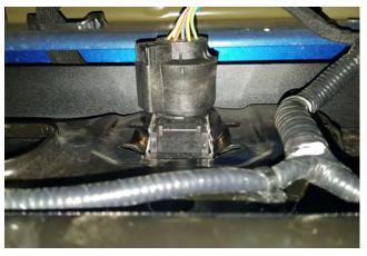
**STEP 1** // Unplug the factory license plate lights harnesses and trailer plug connector (if equipped) and pull away from the bumper.
