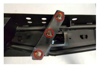
**STEP 7** // If your vehicle is not equipped with a trailer hitch receiver, install the factory triple bolt plate through the back of the mounting tab using the (6) plastic bolt holders.
