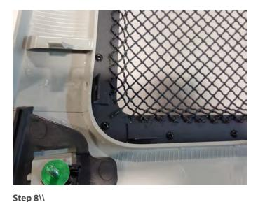
Next, lay the new cutout grille on the factory grille and mark your (12) holes using a marker. Using a 5/16 drill bit and drill, drill out your holes. Then install the (12) M4 screws and nuts securing the grille to the frame.
