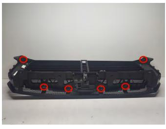
**Step 6\\**Remove the factory grille by removing the (4) push clips on the top, and (2) 8mm screws on the bottom.
