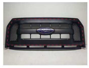
**Step 7\\**Mark and cut out your factory grille using a rotary tool as shown above.
