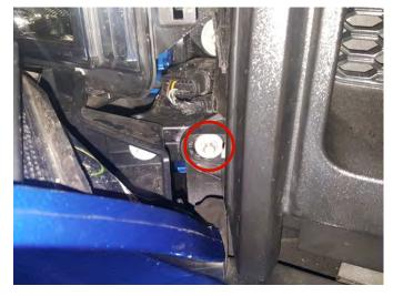
**Step 4\\**Carefully pull back on the headlight trim, and remove the (2) 8mm bolts holding the grille in.
