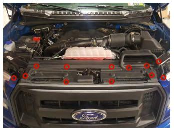
**Step 1\\**Using a panel removal tool, remove the (12) push clips holding the plastic radiator cover to the grille.
