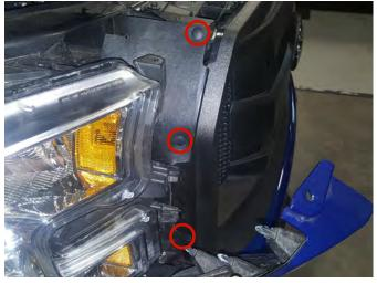
**Step 5\\**With a panel removal tool, remove the (6) push clips holding the side cover in place. Then remove the grille completely from the vehicle.
