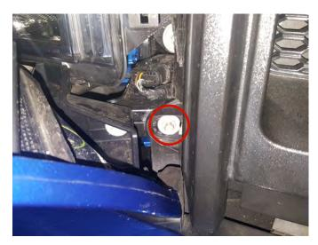
**Step 4\\**Carefully pull back on the headlight trim, and remove the (2) 8mm bolts holding the grille in.
