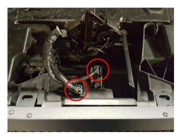
**Step 3\\**Unplug the (2) wire connections by the hood latch.
