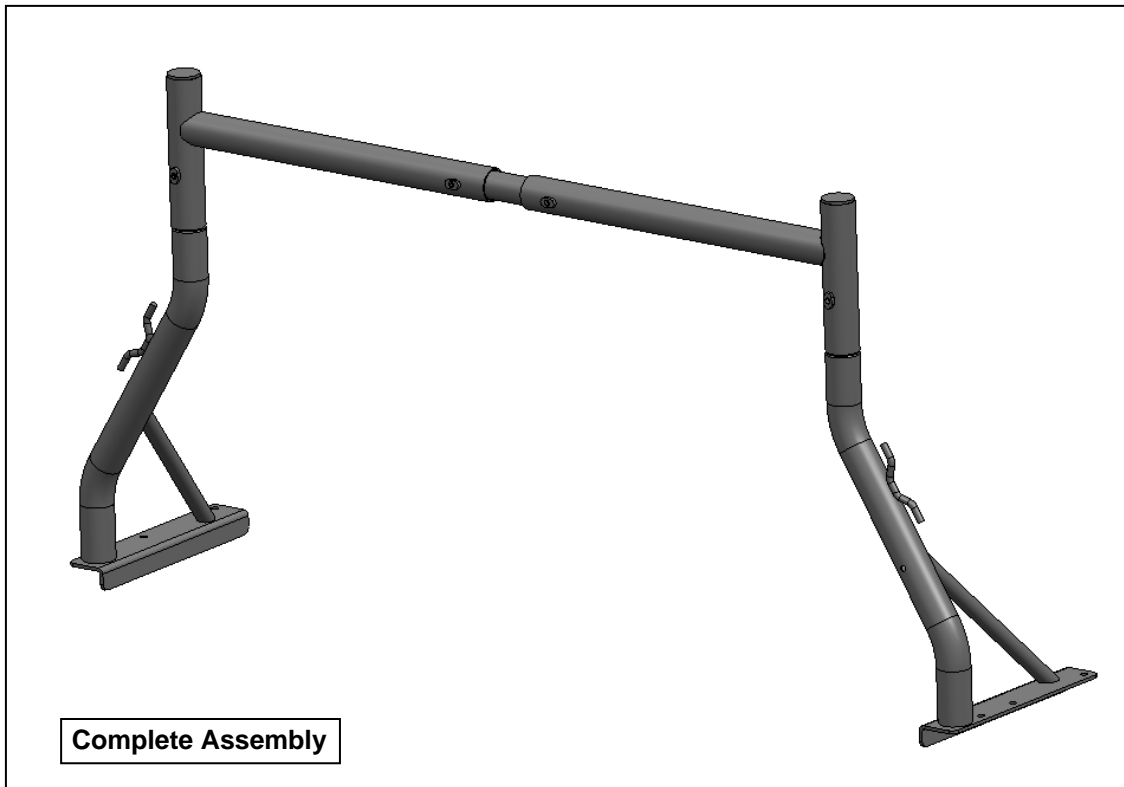
(Fig 4) Tighten the Crossbrace with Allen Head Set Screws
