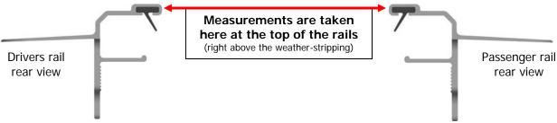
**STEP 9 a.** Measure and record the distance between the rails at A - next to front cover screws. This is your base measurement.
