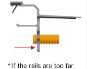
apart, turn the adjustment screws in. (clockwise)
