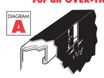
For each clamp mark on your bedliner a 1-1/2" x 3" hole as shown above. Remove clamp. Cut holes in bedliner. Reinsert side rail clamp. Return to step 6.
