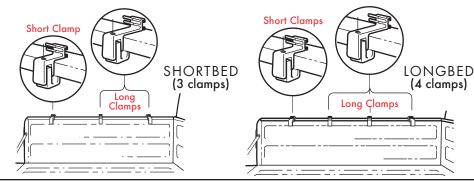
**Longer Clamps** Some trucks use different sizes of clamps to fit curved sidewalls. Longer clamps go in the forwardmost (Cab) positions while the shorter clamps hold the rails at the rear (tailgate) end.
