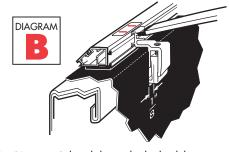
Side rail clamped to bed with bow attached.
