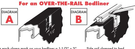
For each clamp mark on your bedliner a  $1-1/2" \times 3"$ hole as shown above. Remove clamp. Cut holes in bedliner. Reinsert side rail clamp. Return to step 5.
