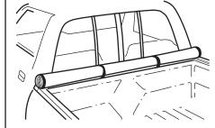
EASY USE OF TRUCK BED Tarp may be rolled up and secured with Velcro® for bulk hauling
