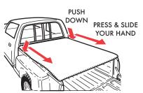
D. Finish attaching tarp along each side by pushing down and sliding you hand towards each corner. You can feel the "grip" action.
