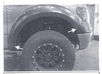
**STEP 3:** Place the Fender Flare onto the vehicle and fit into the correct position following the contours of the body. Use four (4) of the .6mm clips (two (2) per side) to secure the Fender Flare to the body. Make sure the dimple in the clip securely attaches in the slot on the Fender Flare.
