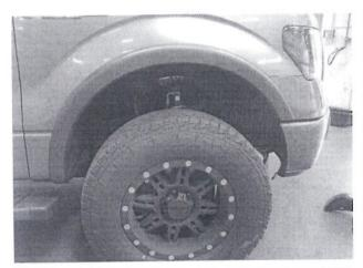
**STEP 1:** Clean the body areas where the Fender Flares will make contact using a clean cloth.
