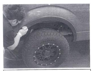
**STEP 7:** Clean the body areas where the Fender Flares will make contact. Use the supplied alcohol wipe.
