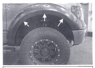
STEP 4: Insert six (6) of the .9mm lever retaining clips (three (3) per side) into the Fender Flare. Make sure the tab in the clip securely attaches in the slot on the Fender Flare. Secure with four (4) bolts removed in Step 6. For 2007-2013 vehicles, secure the center clip with the included scrivet.
