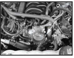
Step 9 Install the coupler on the throttle body and secure the coupler in place. Install a second clamp but do not tighten at this time.
