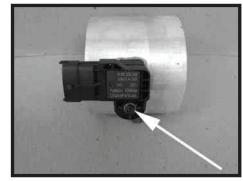
Install the pressure sensor into the intake tube with the supplied hardware.
