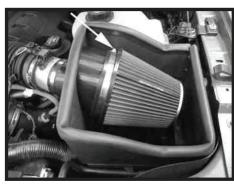
Install the supplied air filter and clamp and tighten the clamp that secures the air filter. If needed, rotate the air filter/velocity stack adapter assembly for the maximum clearance as shown.
