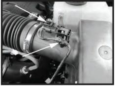
Step 2 Disconnect the electrical connector at the pressure sensor tube to the air box lid. and unclip the wiring harness from the stud.
