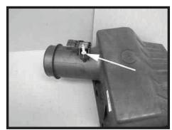
Step 5 Remove the pressure sensor from the factory intake tube.
