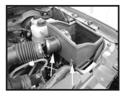
Step 8 Install the heat shield making sure that the tabs on the heat shield are inserted into the lower factory airbox slots. With the heat shield located into the slots, using the 2 factory clips from the airbox, clip the heat shield into position. The center clip will not be used and can be removed if desired.
