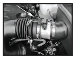
Step 10 Reconnect the pressure sensor electrical connector.
