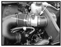
Step 9 Install the intake tube into the coupler on the heat shield then into the stock intake tube. Fasten securely in place.
