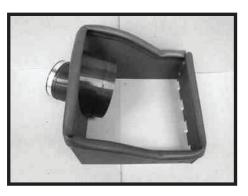
Step 7 Assemble the heat shield with the tabs placed on the inside of the heat shield. Install the rubber bulb seal. Place the velocity stack adapter in the heat shield and install the supplied angled coupler making sure the coupler is pushed completely against the heat shield. Take note of the orientation of the funnel, this may be rotated slightly once the filter is installed in the vehicle. Once the adapter and coupler are tight against the heat shield, tighten the clamp.
