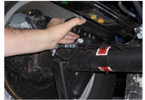
Lower axle enough to remove factory block.
