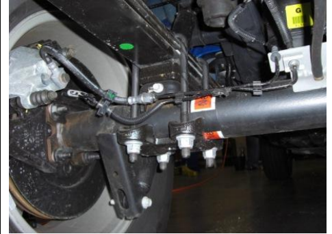
View of 4WD rear axle and leaf spring, note factory block
