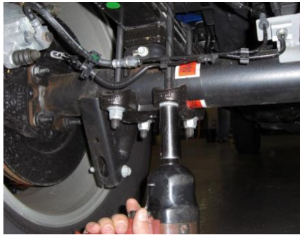
Loosen and remove factory u-bolt hardware.
