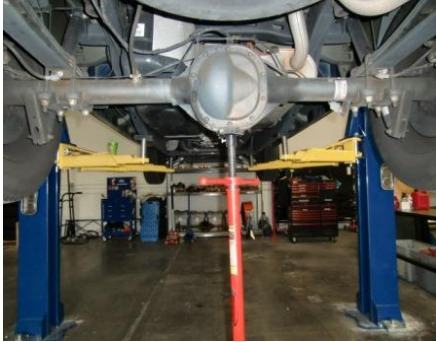
Raise vehicle securely by frame and support axle with jack..
