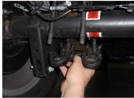
Remove u-bolt nuts and lower plate.
