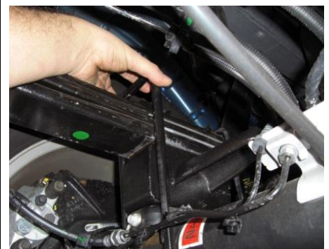
Slide new u-bolts over leaf pack and bump stop bracket.
