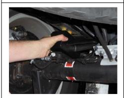
Install lift block with centering pin toward axle.
