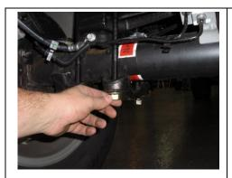
Attach lower mounting plate with provided hardware.
