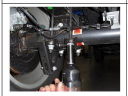
Loosen and remove factory u-bolt hardware.
