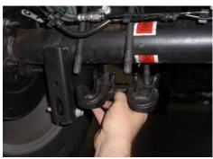
Remove u-bolt nuts and lower plate.
