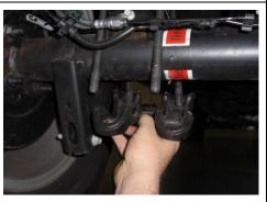
Remove u-bolt nuts and lower plate.
