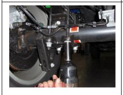
Loosen and remove factory u-bolt hardware.
