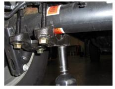
Snug hardware down, lower vehicle on ground and torque.
