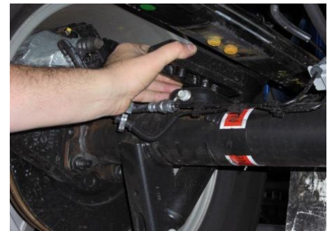
Lower axle enough to remove factory block.
