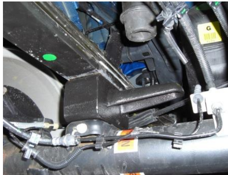
Raise axle and ensure locating pins are properly aligned.
