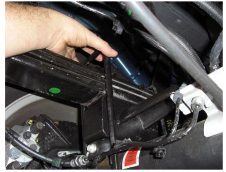
Slide new u-bolts over leaf pack and bump stop bracket.
