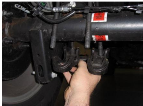
Remove u-bolt nuts and lower plate.
