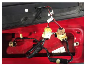
**Step 3\\**Take the new Axial light, and install the two light harnesses into the factory light bulb sockets. Install the brake light wire into the middle socket. The cab light can be installed into either end socket. Test for proper function.
