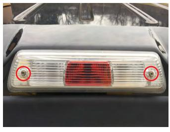
**Step 1\\**Locate, and remove the (2) phillips head screws.
