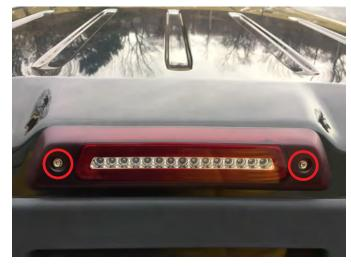
**Step 4\\** Install the (2) factory screws and tighten fully.
