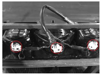
**Step 2\\**Remove the (3) light bulb sockets by twisting them counter clockwise. Then remove the (3) bulbs by gently pulling away from the socket.
